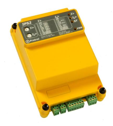
IPS2 is a fault passage indicator for overcurrent and earth faults that signals using both its relay output and an optional external LED. Powered by internal supercapacitors, it provides local indication using the external LED for 24 hours.
