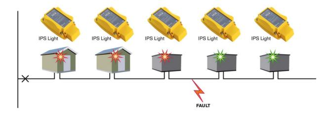
The stations "upstream the fault" are flashing red, while those "downstream the fault" are flashing green. The repair personnel can thereby easily and fast localize the fault on the cable.
